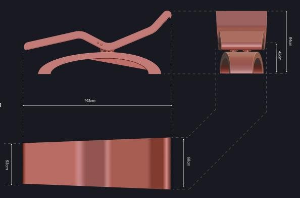
General protection: Temperature: Heated area standard: Heating system standard: Voltage standard system: Thermostat: Power outlet: Lift for automatic tilting: Certifications: IP54 - IP67 Up to 41.5°C/105°F 1 zone holohedral Electric space heating cables 220-240V/800W; 110-120V/950W Digital; IP65 UL-TÜV approved European Bosch standard ; IP54 Linear actuators; UL-TÜV approved; IP65 UL-TÜV approved components
